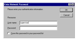
Type **supervisor** in the **User Name** field (no password needed) and click **OK**. The **Firewall Configuration** screen is displayed.
